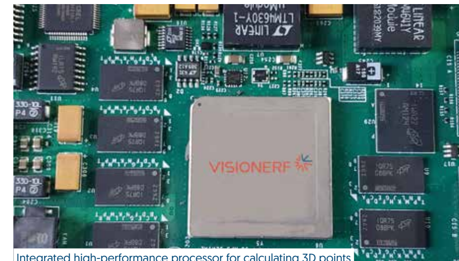
Integrated high-performance processor for calculating 3D points
